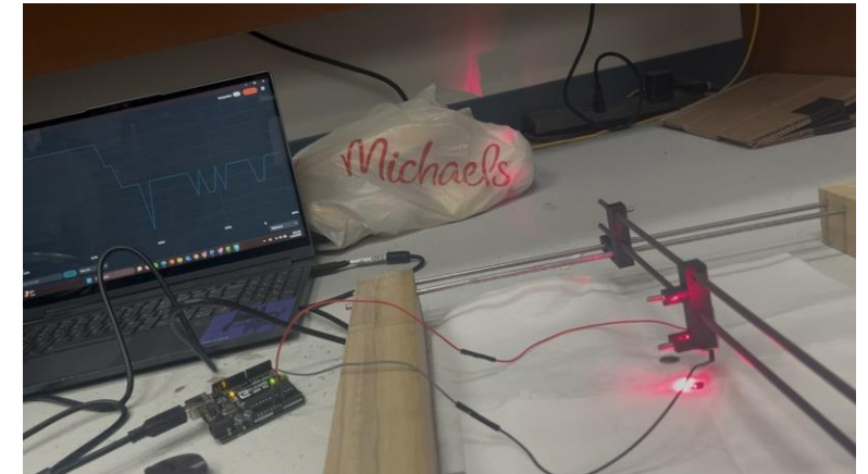
Demonstration of a BPW34 photodiode detecting scattered reflections from a red test laser. The voltage reading significantly drops when beam is moved from the white fabric onto the black spot.
